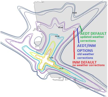
Noise Contour Differences due to Atmospheric Absorption
