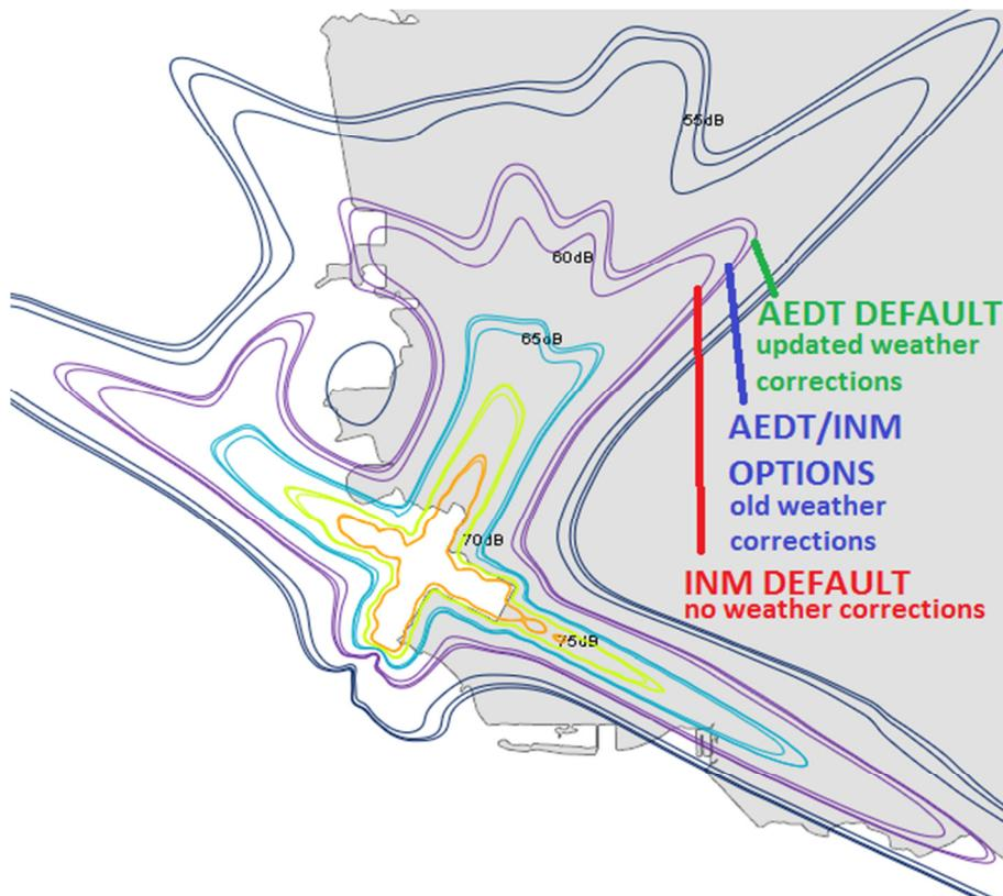
**Noise Contour Differences due to Atmospheric Absorption**
