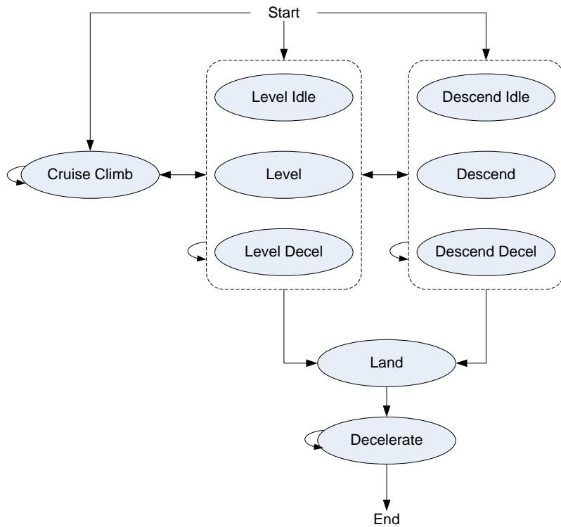
Figure 1: Airplane Approach Step Transition Diagram
