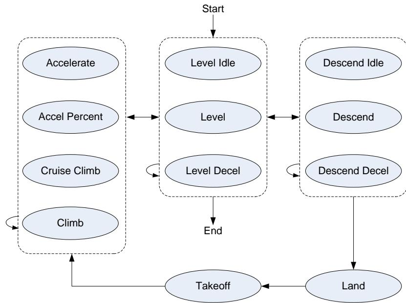
**Figure 3: Airplane Touch and Go Step Transition Diagram**
