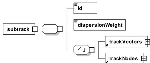
A collection of segments representing a flight track. AEDT 2a only processes the first subtrack associated with a track.
