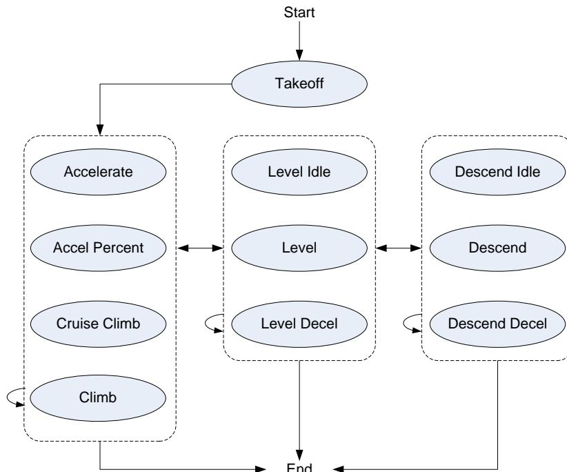
Figure 2: Airplane Departure Step Transition Diagram
