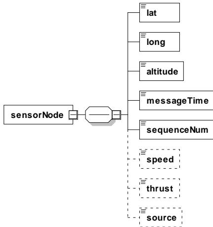
Describes a single node of a radar flight path.
