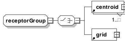
Contains either a centroid or a grid to indicate a location.
