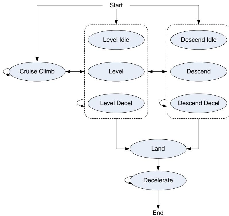
Figure 1: Airplane Approach Step Transition Diagram
