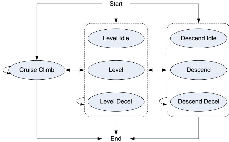
Figure 5: Airplane Overflight Step Transition Diagram
