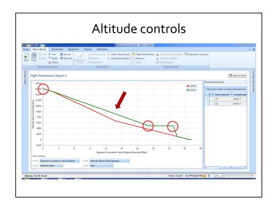
• The fictional green profile has two "At" altitude controls of 5,000 feet, representing an altitude hold near the airport.
