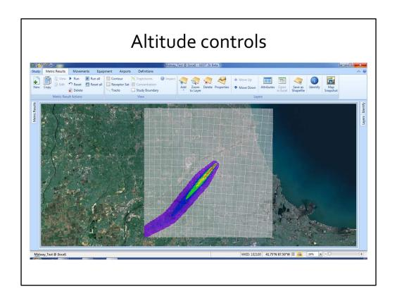
• 300 fictional flights flying in the daytime along the red profile give the colored noise receptor grid shown here.
